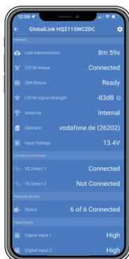
The GlobalLink 520 connects your remote Victron system or individual products to VRM, our online [Victron Remote Management portal](#). Through that portal, you can monitor current and historical system operation – such as battery voltage and state of charge – from anywhere in the world. VRM is free to use.
